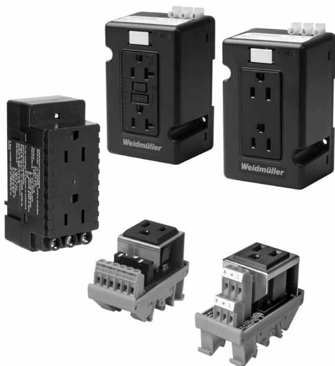
DIN-rail receptacles, 5A, 15A and 20A power outlets, provide a convenient power source for portable computers or test devices for in-the-panel troubleshooting. They mount on standard 35mm DIN-rail. The terminations accept slotted or Phillips screwdrivers. The mounting foot includes a latching lock - slide it open, mount the module on the DIN-rail and slide the lock closed.
