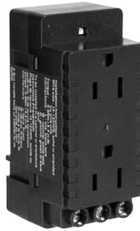
This new DIN-rail mountable duplex receptacle makes adding a 120V maintenance AC outlet to control cabinets quick and easy. It mounts on standard 35mm DIN-rail and requires just 42mm of rail space. An LED indicates that 120V is applied to the module. The terminations accept slotted or Phillips screwdrivers. The mounting foot includes a latching lock – slide it open, mount the module on the DIN-rail and slide the lock closed.
